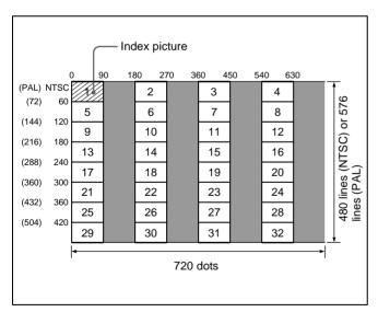
Seven frame spaces are reserved at the end of the last scene as a recording area for index pictures. (A cassette with 16 Kbits of cassette memory can record up to 198 index pictures, and a cassette with 4 Kbits of cassette memory can record up to 45 index pictures.)
